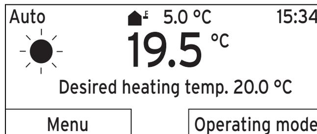
1. If the display does not show the basic display, press the left-hand selection button, **Back**, until the basic display appears again.
